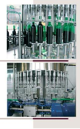
These machines are based on the method of gravitational filling by level under low vacuum. The special design of the filling prevents losing of alcohol degrees or flavours. When working with wine, before the filling starts inert gas is injected into the bottle to eliminate the possibility of oxidation of the wine. To reduce foaming, product flow is adherent to bottles walls. Our production range includes machines with capacity ranging from 800 to 12 000 bottles per hour.
