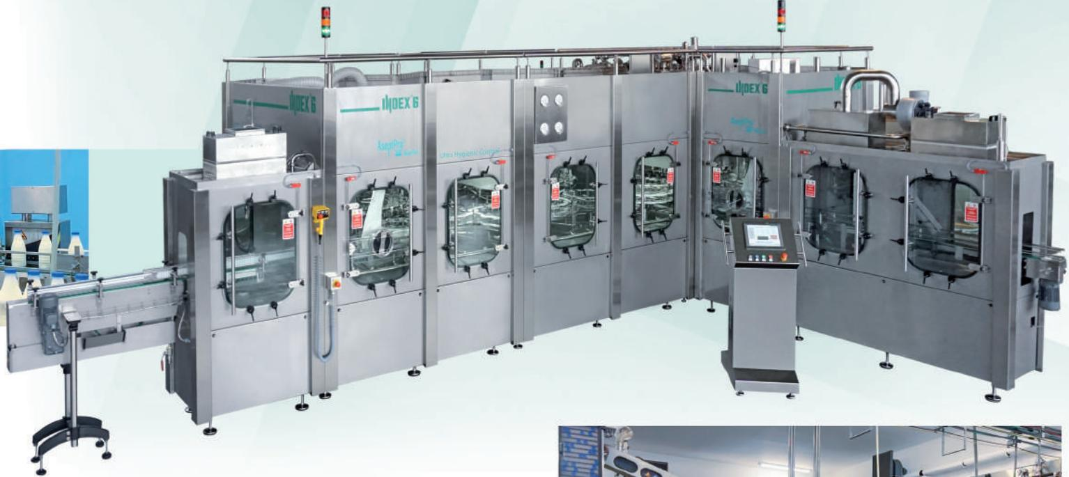
**WET PPA Technology** for bottles decontamination (NO spores).
