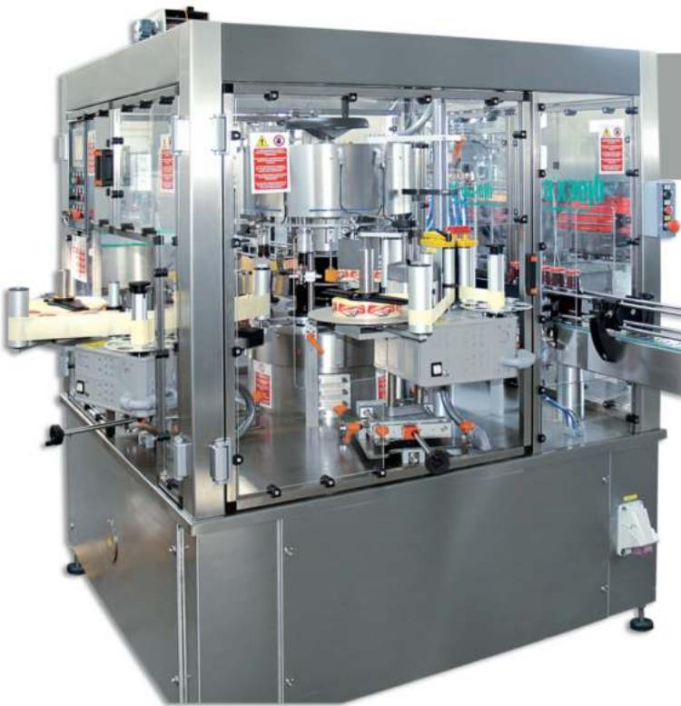
Rotary machines for application of labels on cylindrical, oval, conical and polyhedral containers. Up to five label application modules can be installed.
